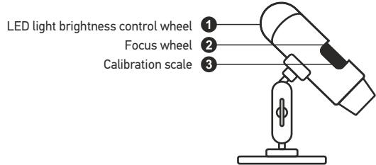
The kit includes: microscope, Discovery Artisan installation CD, calibration scale, user manual.
